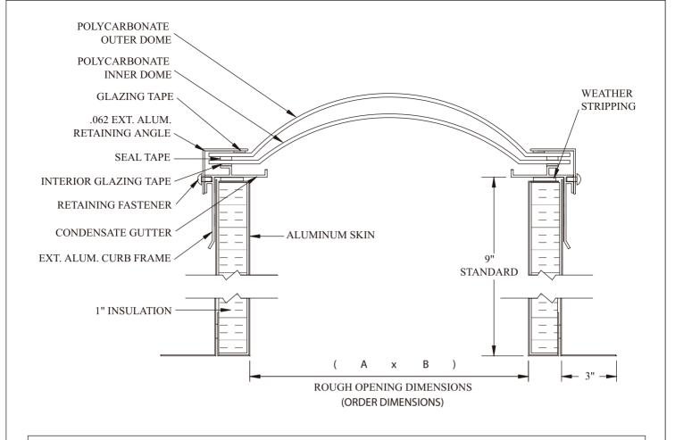
SELF-FLASHING POLYCARBONATE SKYLIGHT, WITH INSULATED CURB - Specification: Self-Flashing Polycarbonate (dome or pyramid as an option) skylights, ORCA Manufacturing, Inc.,
