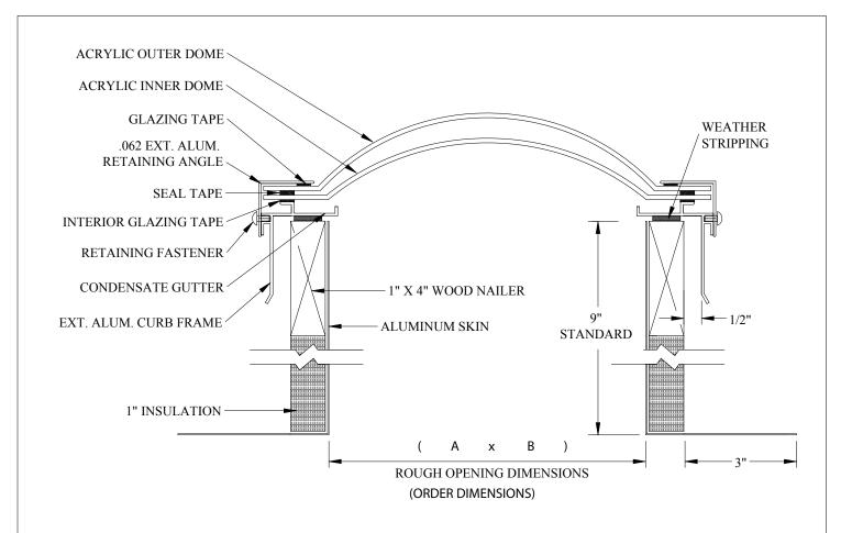
SELF FLASHING ACRYLIC SKYLIGHT - INSULATED CURB with NAILER - Specification:
