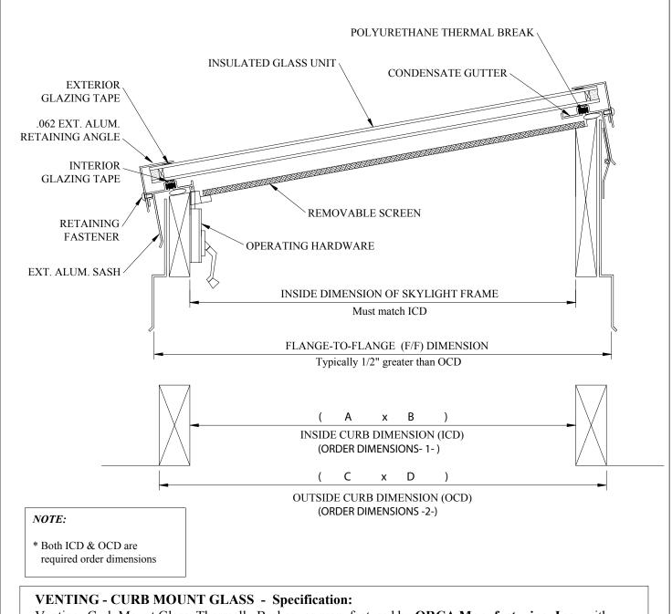
Venting- Curb Mount Glass; Thermally Broken, as manufactured by **ORCA Manufacturing, Inc.,** with insulated glass unit (Clear tempered over tempered standard, Low-E, tinted or laminated as an option) in a welded thermally broken, extruded aluminum sash. Finish in bronze, (or white gloss enamel as an option).
