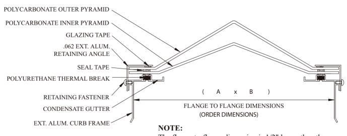
The flange-to-flange dimension is 1/2" larger than the outside dimension of curb, unless directed otherwise
